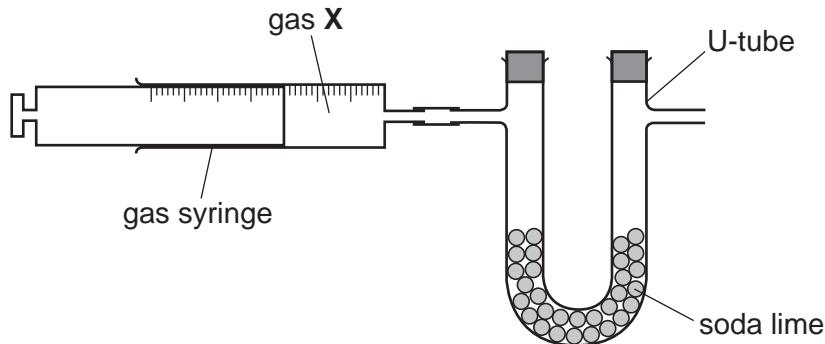
A 100.0 cm<sup>3</sup> sample of pure gas X is placed in a gas syringe. The gas syringe is attached to a U-tube containing small lumps of solid soda lime, a mixture of sodium hydroxide and calcium hydroxide. All of gas X is slowly passed into the U-tube and the mass of gas X absorbed determined.
